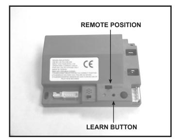
Figure 12.11 Programming RC300AU
